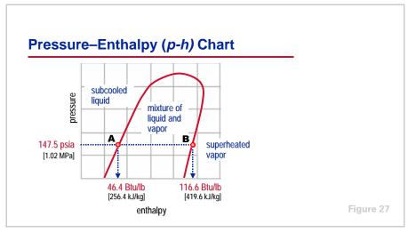
The pressure-enthalpy chart is simply a plot of the saturated properties of a refrigerant. It plots refrigerant pressure (vertical axis) versus enthalpy (horizontal axis). Enthalpy is a measurement of the heat content, both sensible and latent, per pound [kg] of refrigerant.
